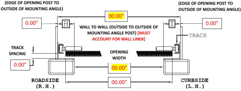
TRANSGLOBAL'S DOOR PANEL WIDTH BASED ON WALL-TO-WALL DIMENSION (IF NOT MOUNTING TRACK AGAINST WALL SPECIFY DIMENSION OUTSIDE TO OUTSIDE OF MOUNTING ANGLE)
